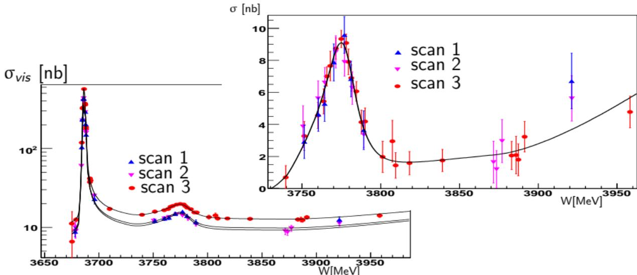
Left: Visible cross section  $e^+e^- \rightarrow \text{hadrons}$  vs. CM energy
