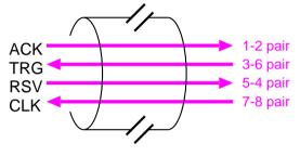
CLK: 127 MHz (derived from 508 MHz RF clock) TRG/ACK: serialized, 254 Mbps
