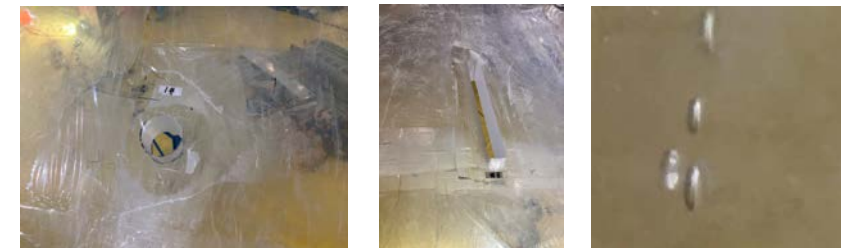
Typical defects to be repaired : holes, rectangles, bubbles. They are mainly from the bonding lines especial the “T” area.
