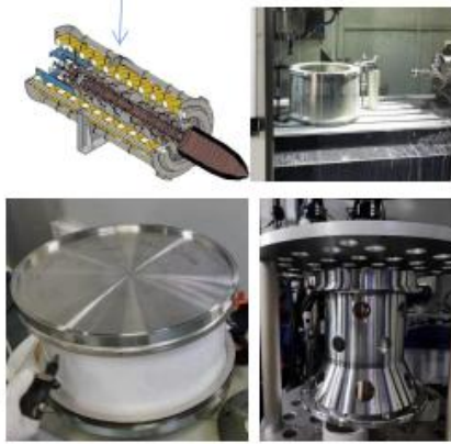
Klystron No. 3 (MB) Efficiency 80.5% (under fabrication)
