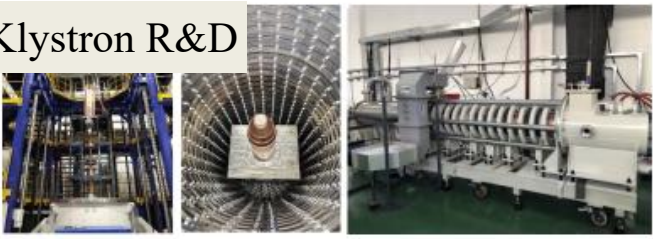
Klystron No. 1 Efficiency 65% (2020)
