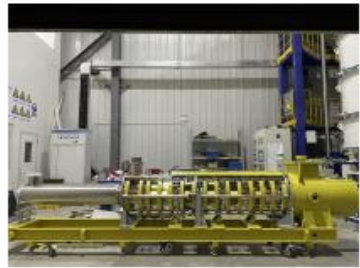
Klystron No. 2 Efficiency 77% (2021)
