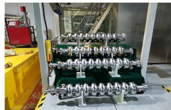
1.3 GHz High Q Mid-T Cavity Horizontal Test
