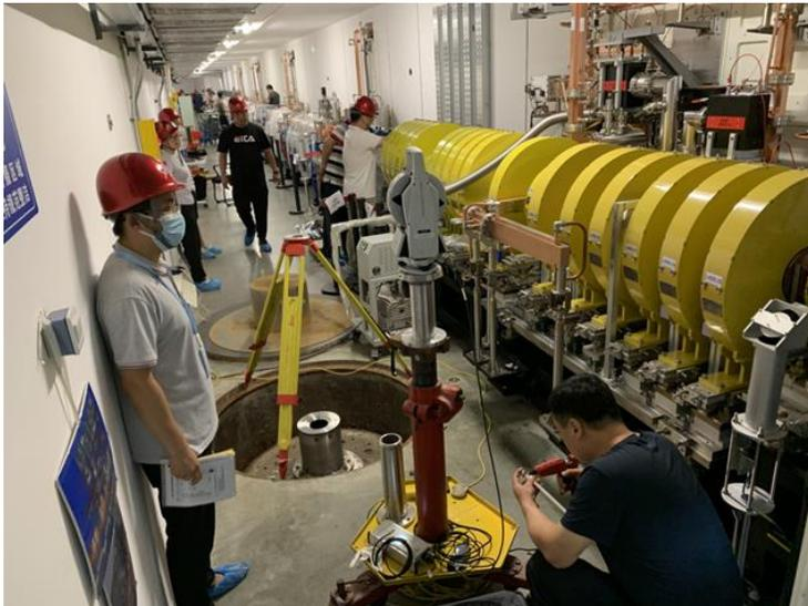
Smooth precise alignment of linear accelerator
