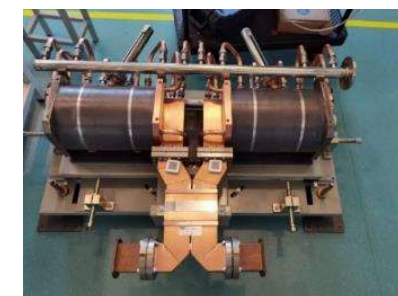
HEPS pulse compressor
