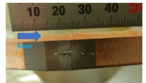
Damaged jaw of D02V1 in LER due to the sudden beam loss
