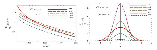
Figure 3. Differential cross section of the process  $pp \rightarrow \text{jet} + Z_{bulk}(\gamma_{bulk})$  for n = 3, 4, 5, 6 at the center-of-mass energy of protons equal  $\sqrt{s} = 14$  TeV. The standard model background is  $pp \rightarrow \text{jet} + \nu\bar{\nu}$ .
