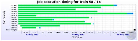
**Figure 6**. Typical ALICE analysis job time profile. The green bars represent the data processing time, the blue bars represent the merging stages per data set (in this case a run), while the final merging stage is the black bar starting as soon as the last merging job per run is completed.
