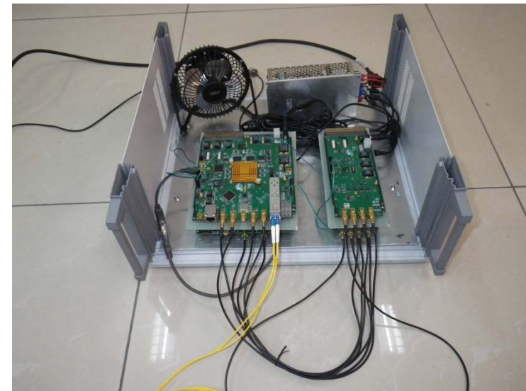
The prototype of the Self-Triggering Front-End Station without the analog front end
