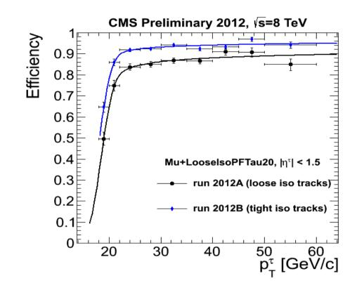
Efficiency measured using tag-and-probe technique with  $Z \rightarrow \tau^+ \tau^-$ ,  $\tau \rightarrow \mu \nu + \tau$ -hadr using an unbiased dataset for the T&P.
