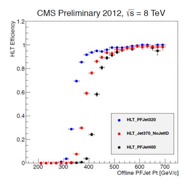
Turn-on cuve measured vs. offline Particle Flow jet pT. Trigger efficiency measured on an unbiased data sample from Run2012C.
