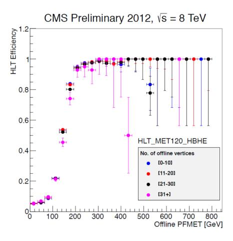
Turn-on curves for HLT\_MET120\_HBHE trigger, in bins of different pileup (based on # offline vertices): PU has no effect on trigger turn-on.
