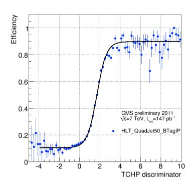
Turn-on curve of the Track Counting High Purity (TCHP) discriminator efficiency at HLT, with respect to the same variable computed offline. The TCHP b-tagging discriminator is the third
