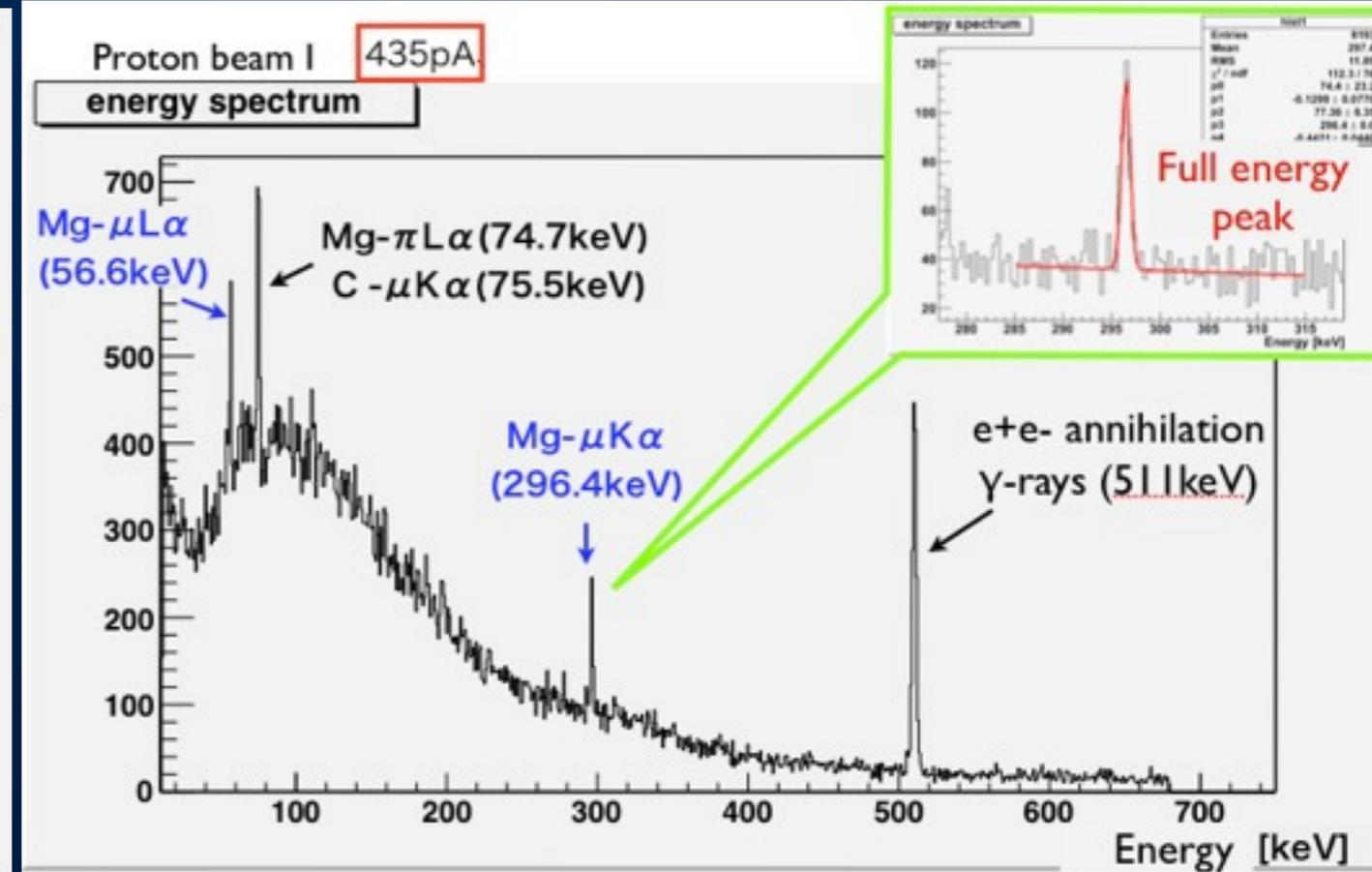
Measured muon yield at the exit of the 36° transport solenoid
