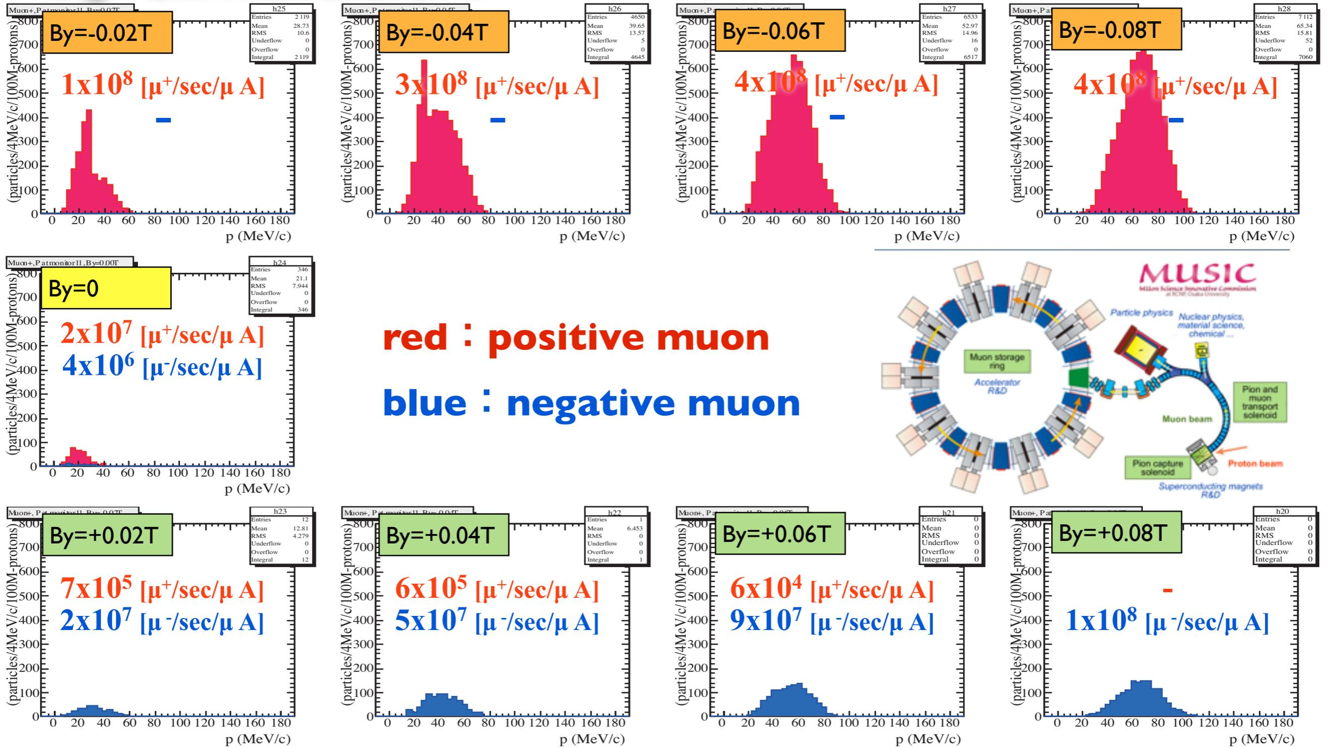
Changing magnitude and direction of the dipole field, we can select charge and momentum of the beam.
