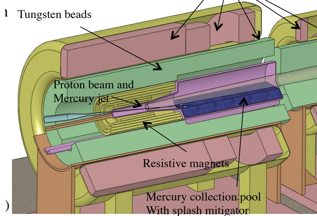
5-T copper magnet insert; 10-T Nb3Sn coil + 5-T NbTi outsert.
