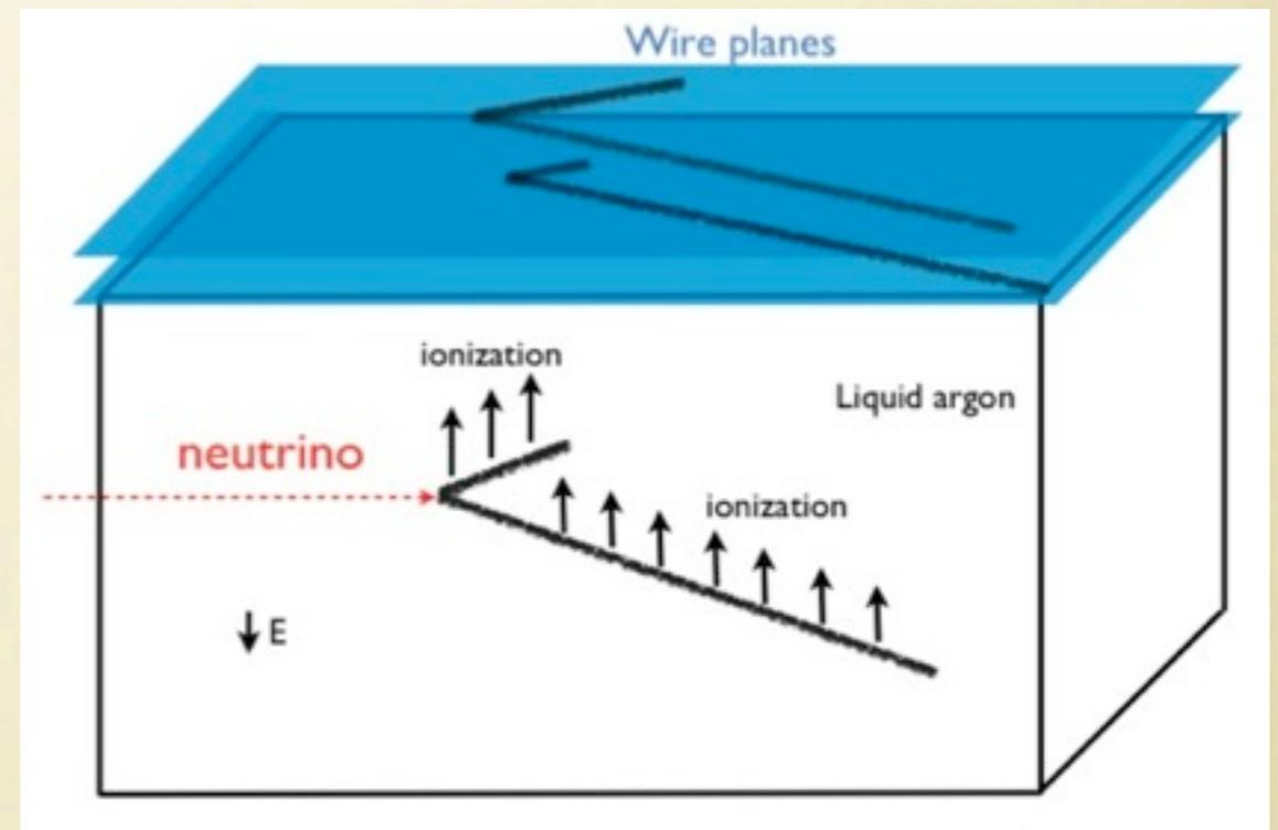
Ref: *The Liquid-argon time projection chamber: a new concept for Neutrino Detector*, C. Rubbia, CERN-EP/77-08 (1977)
