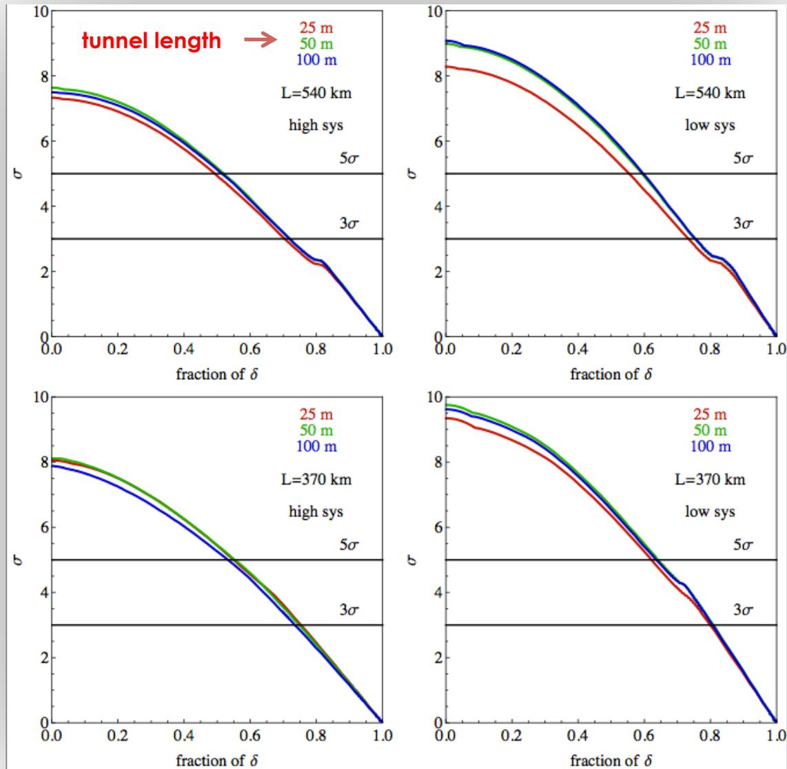
No significant increase in physics performance by using lengthier decay tunnel
