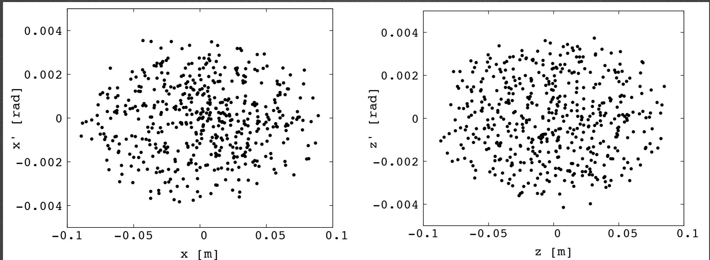
Injected Beam in the horizontal (left) and vertical (right) phase spaces
