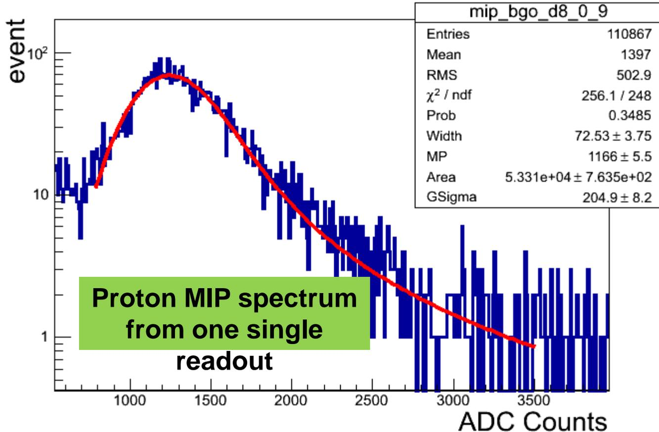
Fitting Function: Gaussian convolution
