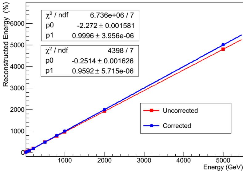
**Leakage Correction can also give a better linearity. The gradient from 0.9592 to 0.9996. We wish it perfectly equal to 1.**
