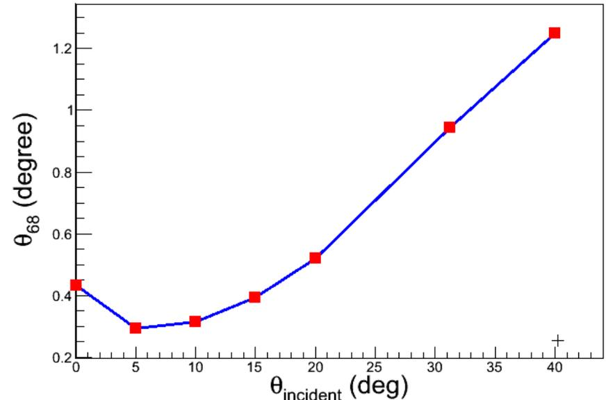
**Angle resolution for electrons as a function of energy and angle**
