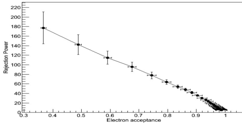
Neutron detector rejection power depending on electron selection eff.
