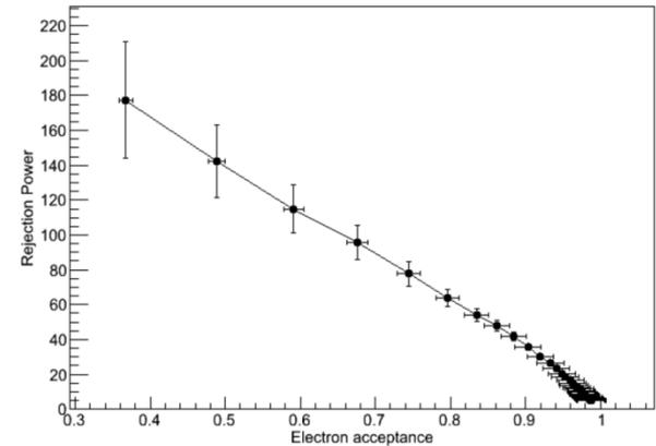
Neutron detector rejection power depending on electron selection eff.
