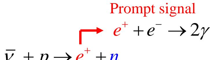
Delayed signal, Capture on H
