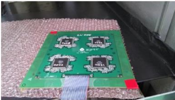
readout electronics board 16 \times 16 \text{cm}^2
