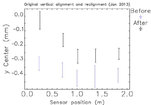
Figure 15: Vertical center of chamber with respect to the user beam orbit. Sensors 2-6, January 2013 data.
