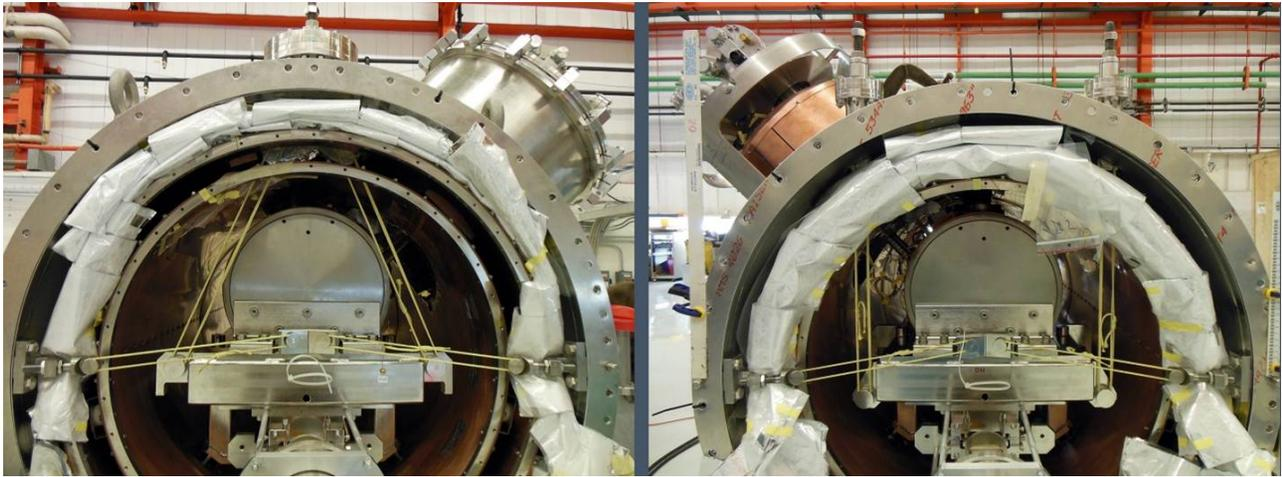
Figure 6: Kevlar band suspension system.
