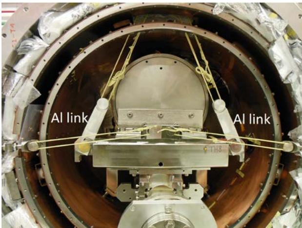
Figure 11a: Kevlar with added aluminum links suspension system (upstream end).
