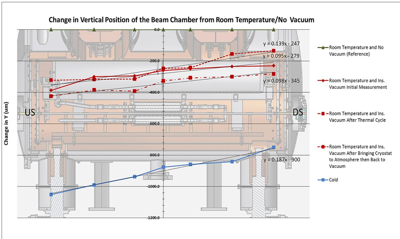
Figure 10: Vertical position of the cold mass during the cool down cycle.
