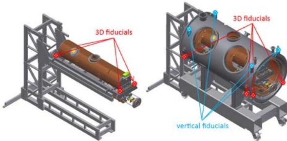
Figure 7: Vacuum vessel is moved into the cold mass and aligned.
