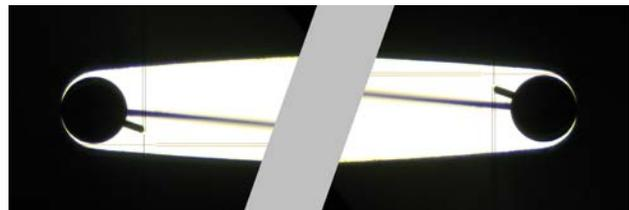
Figure 9: Spherical target inside the prototype of the SCU0 vacuum chamber photographed through the alignment scope of the optical level.
