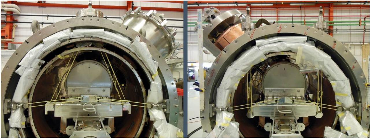
Figure 6: Kevlar band suspension system.
