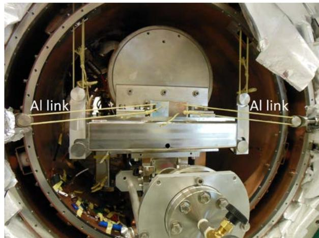
Figure 11b: Kevlar with added aluminum links suspension system (downstream end).
