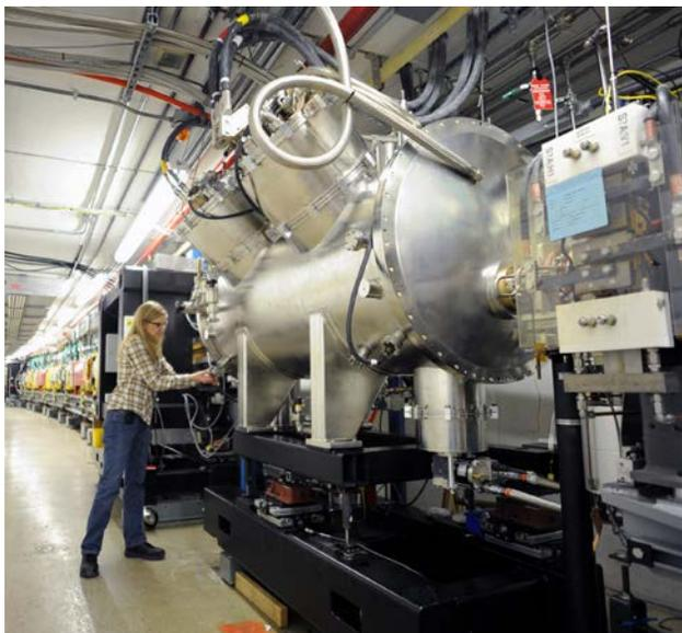
Figure 13: APS storage ring with the SCU0 installed.
