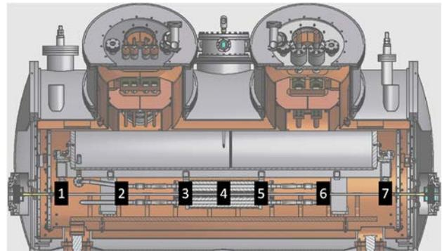
Figure 8: Position of bead targets inside the chamber.
