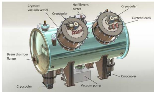
Figure 1: Cryostat
