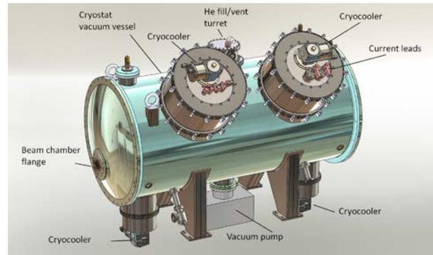
Figure 1: Cryostat
