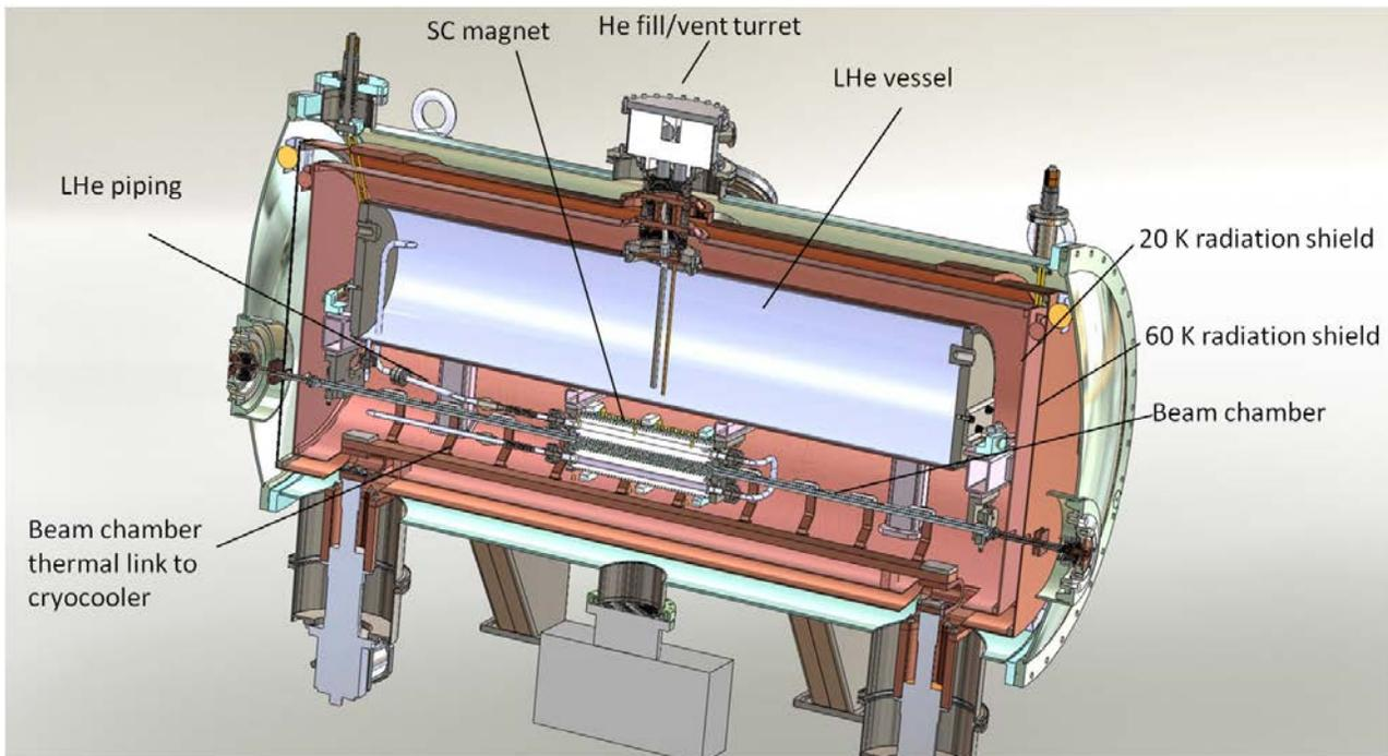
Figure 2: Cutaway view of the inside of the cryostat.
