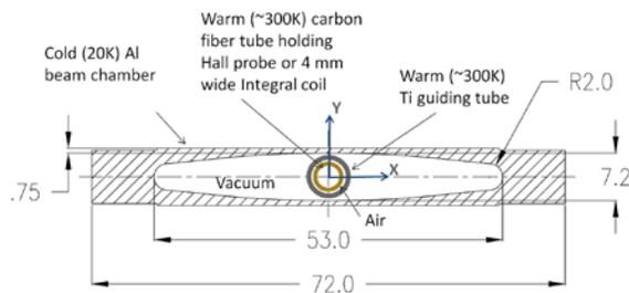
Figure 12: Magnetic mapping of SCU0.
