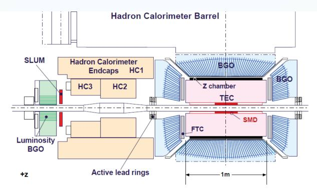
Figure 1: Side-view of the central region of the L3 experiment on the +z side, showing the beam pipe and the position of the luminosity BGO calorimeter and the silicon tracker (SLUM).
