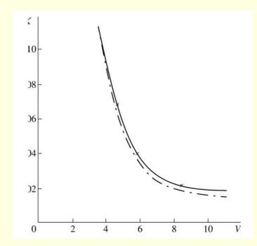
Figure 2: Frequency-contrast characteristic of an optical channel with a deflecting mirror:
