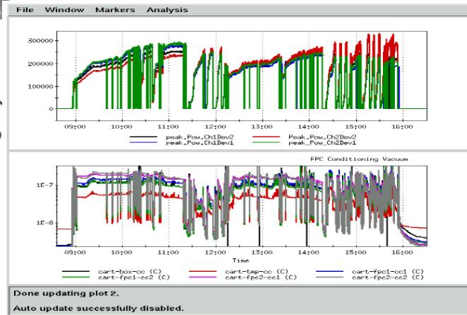
Figure 7: Typical vacuum trip during conditioning.
