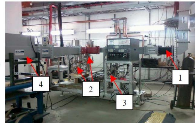
Figure 5: Assembly of the FPCs for conditioning.
