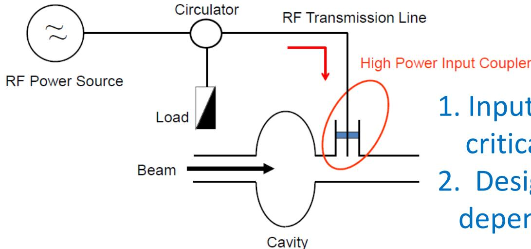
1. Input coupler is one of the most critical component of an SRF system.
