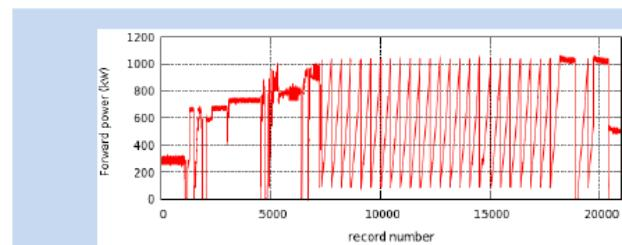
Test of the HIPPI power coupler on the HIPPI cavity at 1.8 K, full reflection
