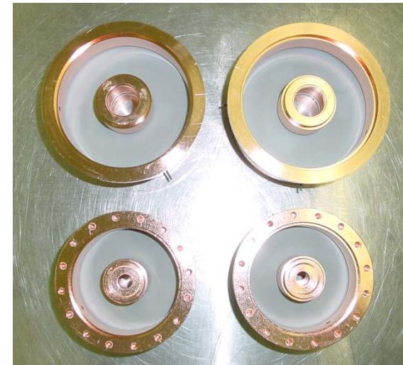
$\text{Al}_2\text{O}_3$  ceramics with metalizing
