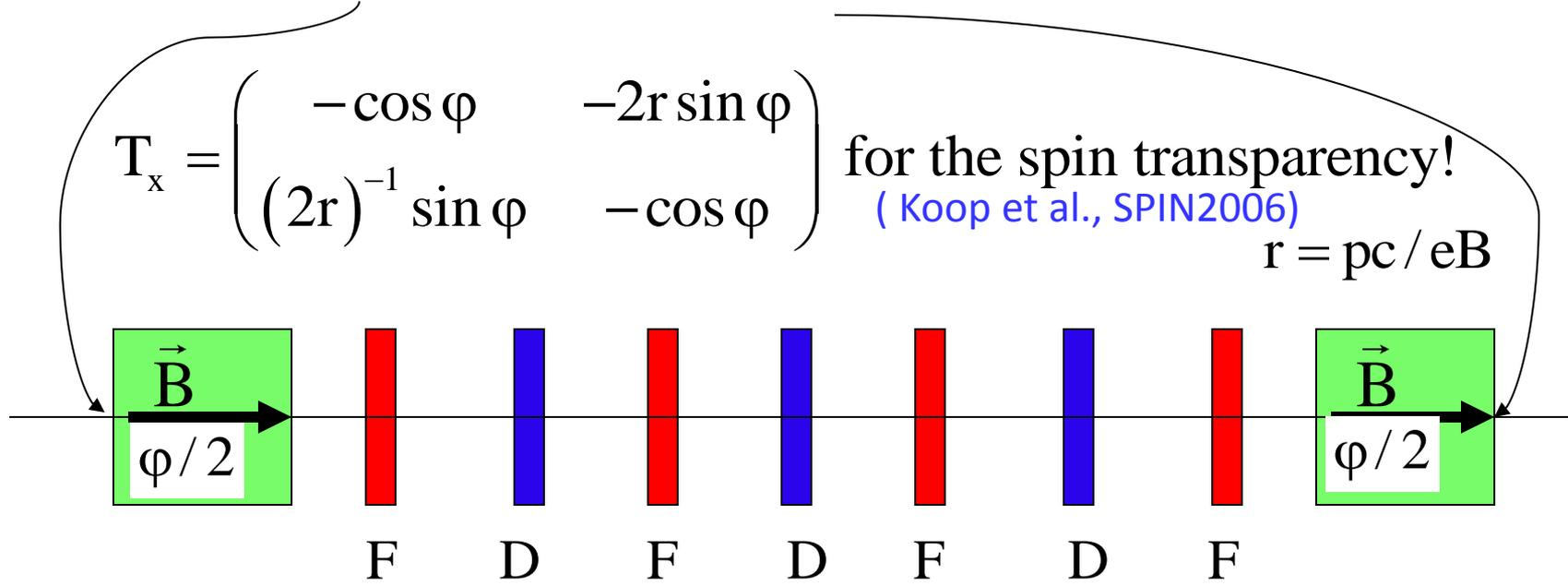
Two solenoids, each  $L=40\text{ m}$   $B=5\text{ T}$ , provide spin rotation by  $\varphi = 180^\circ$  at  $E=45.5\text{ GeV}$ . Extension to  $120\text{ GeV}$  with  $B=10\text{ T}$  looks feasible.
