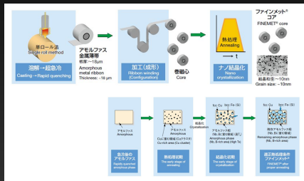
Production process of finemet cores.
