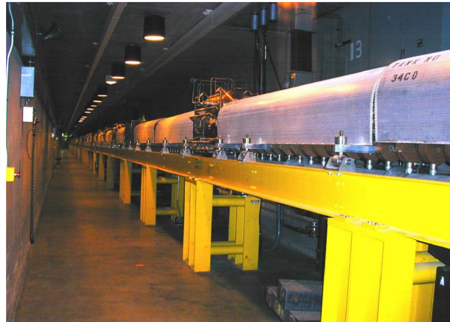
805MHz SCL linac of 800 MeV with 44 modules
