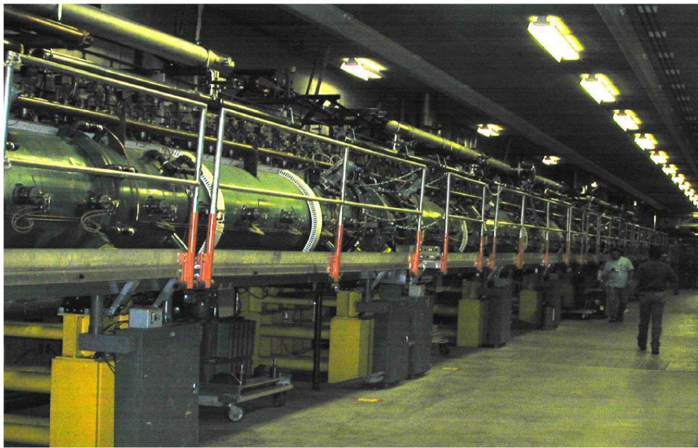
Four 201.25-MHz drift tube linac (DTL) tanks accelerate beam from 750 keV to 100 MeV
