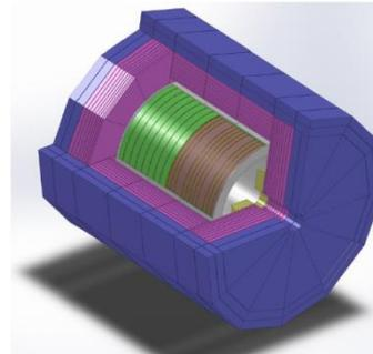
Structure of the coil/iron yoke
