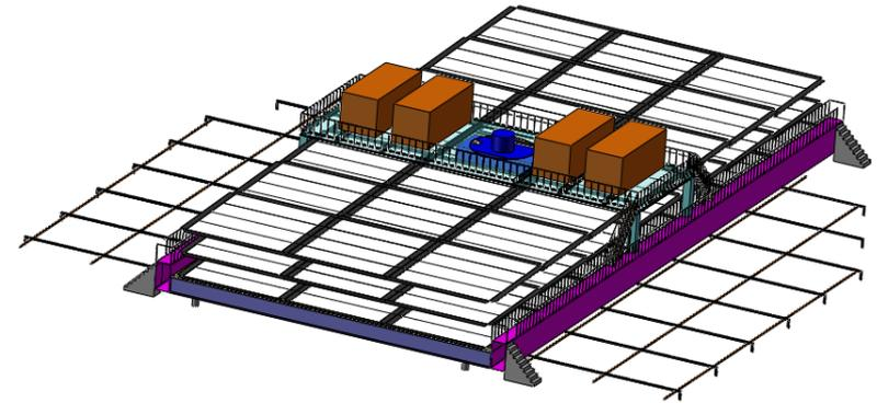
The Target Tracker consists of several wall. Each wall consist of 4 modules in horizontal position and 4 modules in vertical position, allowing a good tracking reconstruction capability.
