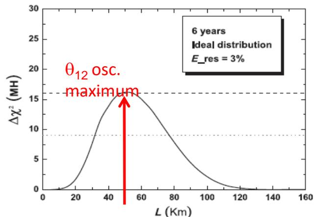
Multiple reactors cores may reduce the MH sensitivity (Baseline difference can not be more than 0.5km)
