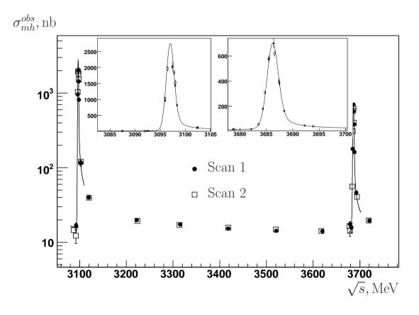
KEDR scanned  $\sqrt{s}$  between  $J/\psi$  and  $\psi(2S)$  with 1.4 pb<sup>-1</sup> selecting  $(2-3)\cdot 10^3$  m/h events per point,  $\sim 18\cdot 10^3$  in total V.V. Anashin et al., Phys. Lett. B753, 533 (2016)
