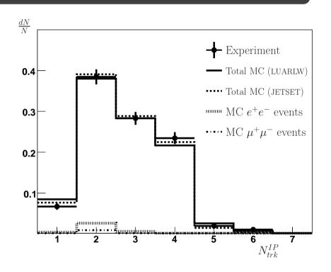
The number of tracks from the common vertex in the IP, Fair agreement of simulation with data ( $\sqrt{s} = 1.94$  and 2.14 GeV)
