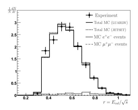
Energy deposited in the calorimeter, Fair agreement of simulation with data ( $\sqrt{s}$  =1.94 and 2.14 GeV)
