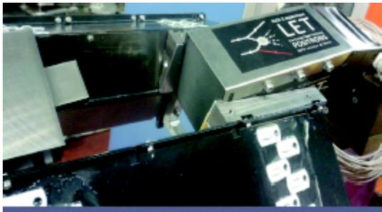
LET station (LYSO crystals) @ 2 m from the IP, in one of the QCALT wedges
