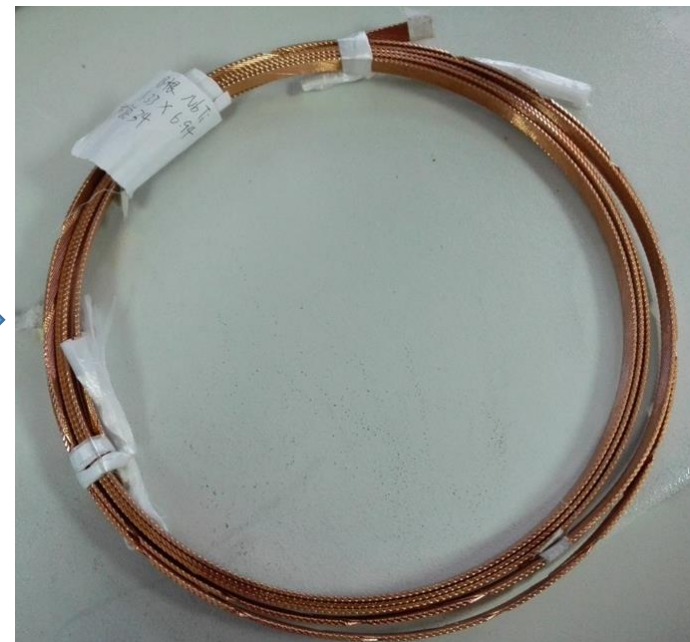
Number of strands : 18 Strand diameter : 1.2mm Materiel :Nb/Ti Complete time:2016.2
