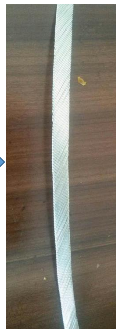
Number of strands : 24 Strand diameter : 0.727mm Materiel :Nb/Ti Complete time:2015.8
