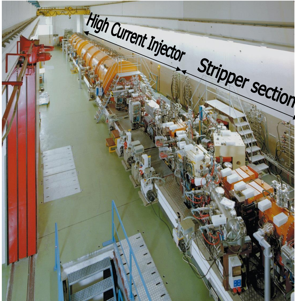
High current injector [HSI]: RFQ and IH structures by Ulrich Ratzinger RFQ renewed by Stepan Yaramyshev
