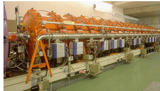
Excellent performance for more than 30 Years, meanwhile problems with cavity cooling and vacuum
