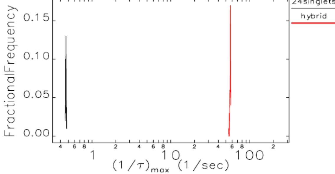
Histogram of possible longitudinal growth rate from four 3 cell cavities.
