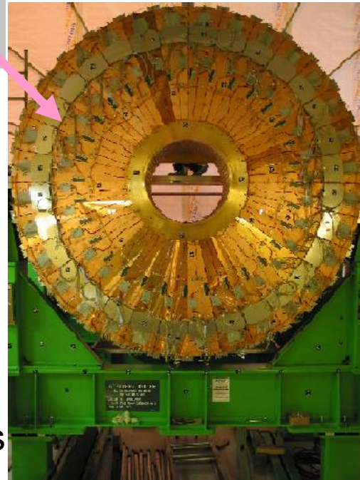
Accordeon shaped interleaved absorber plates and readout boards in liquid argon
