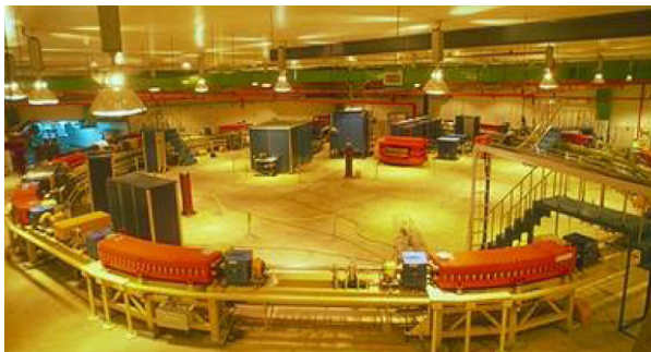
An example of strong focusing synchrotron
