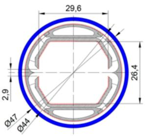
**First FCC-hh beam screen prototype** Testing 2017 in ANKA within EuroCirCol
