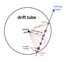
From the ordered sequence of the electrons arrival times, considering the average time separation between clusters and their time spread due to diffusion, reconstruct the most probable sequence of clusters drift times:  $\{t_i^{cl}\}$   $i=1,N_{cl}$
