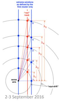
For any given first cluster (FC) drift time, the cluster timing technique exploits the drift time distribution of all successive clusters  $\{t_i^{cl}\}$  to determine the most probable impact parameter, thus reducing the bias and the average drift distance resolution with respect to those obtained from with the FC method alone.
