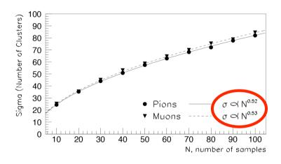
The data taken with a beam of  $\mu$  and  $\pi$  at 200 MeV/c momentum at PSI, refer to a gas mixture He/iC<sub>4</sub>H<sub>10</sub>=95/5, N<sub>cl</sub> = 9/cm, 100 samples, 2.6cm each at 45° (to avoid space charge effects), for a total track length of 3.7 m. A 25  $\mu$ m sense wire (gas gain 2x10<sup>5</sup>), readout through a high bandwidth (1.7 GHz, gain 10) preamplifier, is digitized with a 2 GSa/s 1.1 GHz, 8 bits digital scope. (*NIM* A386 (1997) 458-469 and references therein)
