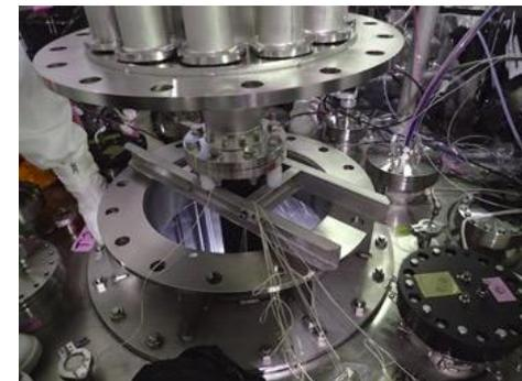
30 m<sup>3</sup> LS w/o Xe has been installed into inner balloon. Now measuring background.
