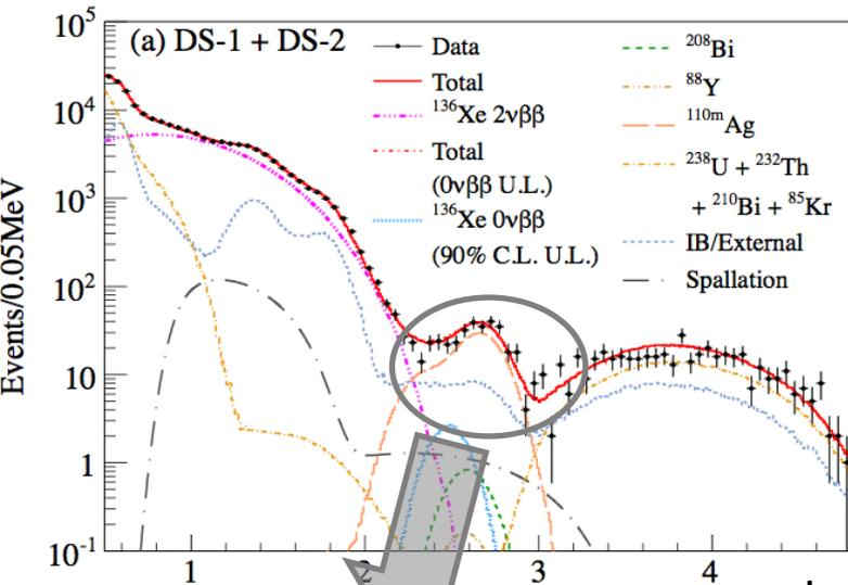
From ENSDF database candidates are  $^{110\text{m}}\text{Ag}$ ,  $^{88}\text{Y}$ ,  $^{208}\text{Bi}$ ,  $^{60}\text{Co}$
