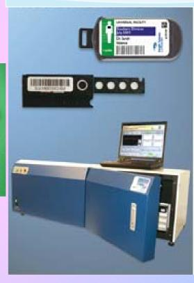
**OSLD** (optically stimulated luminescence detector) make of carbon-doped aluminum oxide  $(Al_2O_3:C)$  which is mainly used for  $\gamma$  and X-ray detection.
