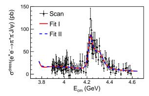
FIG. 1: Measured dressed cross section  $\sigma^{\rm dress}(e^+e^-\to \pi^+\pi^-J/\psi)$  and simultaneous fit to the "XYZ data" (left) and "Scan data" (right) with the coherent sum of three Breit-Wigner functions (red solid curves) and the coherent sum of an exponential continuum and two Breit-Wigner functions (blue dashed curves). Dots with error bars are data.
