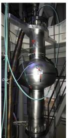
CEPC 650MHz single-cell cavity for vertical test
