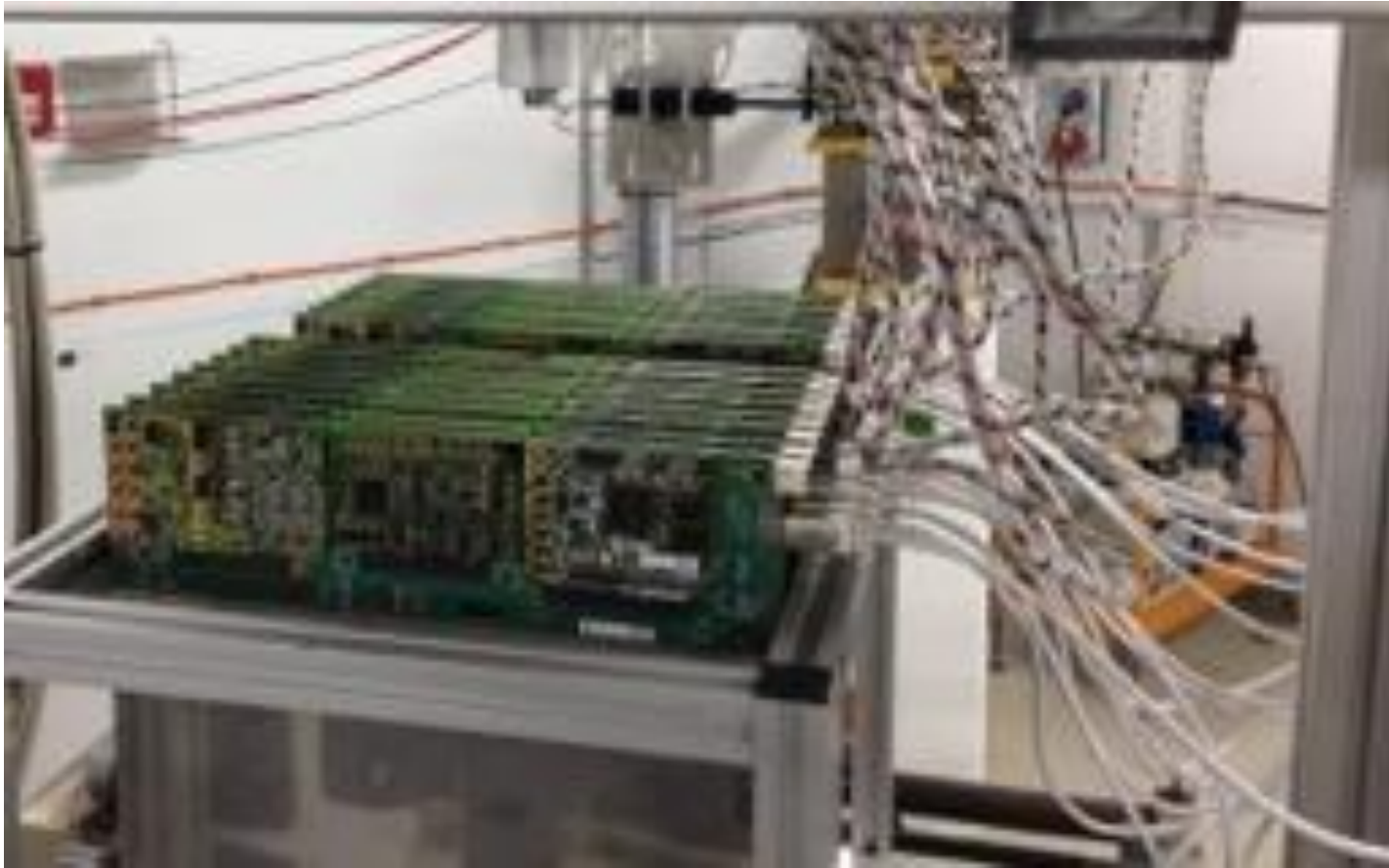
Module 10 layers @DESY Test Beam (electron 1-6 GeV)
