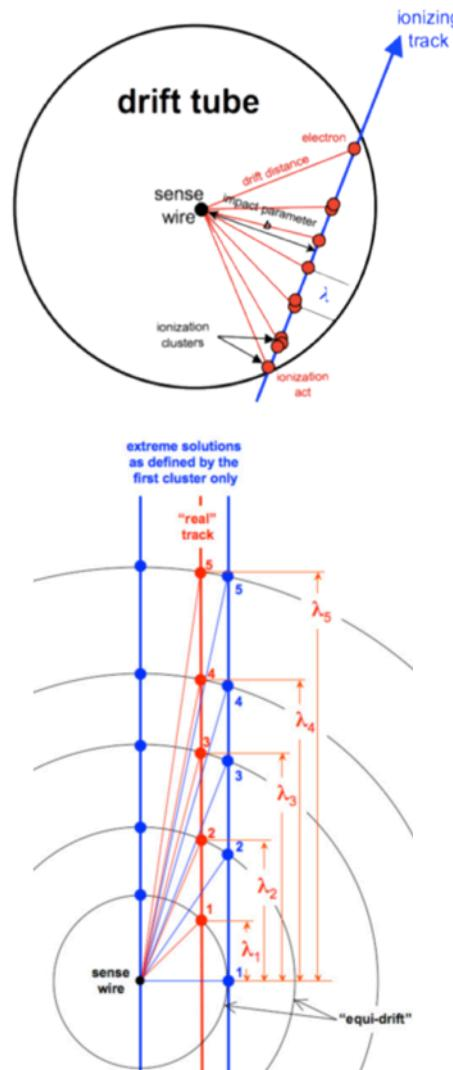
From the **ordered sequence of the electrons arrival times**, considering the average time separation between clusters and their time spread due to diffusion, **reconstruct the most probable sequence of clusters drift times:**  $\{t_i^{cl}\} \quad i = 1, N_{cl}$
