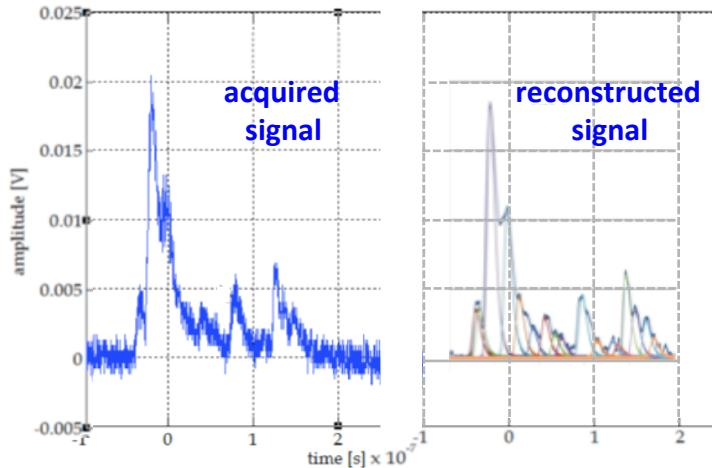
For any given first cluster (FC) drift time, the **cluster timing technique** exploits the drift time distribution of all successive clusters  $\{t_i^{cl}\}$  to determine the most probable impact parameter, thus reducing the **bias** and the **average drift distance resolution** with respect to those obtained from the FC method alone.
