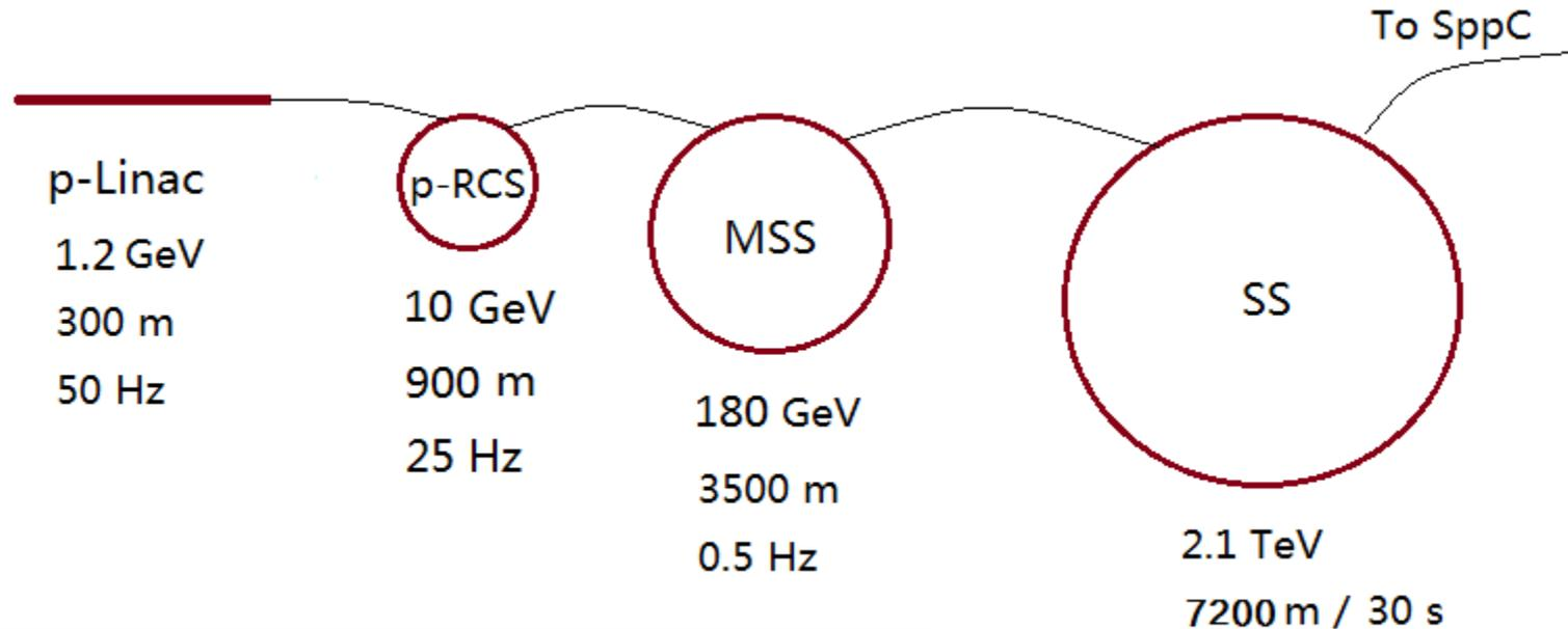
p-Linac: proton superconducting linac
