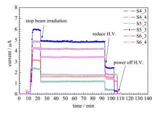
Fig. 6 The current of some cells as a function of time, reaching a maximum of 6 µA due toMalter discharge. The current did not disappear even after stopping beam irradiation, until the high voltage was powered off.
