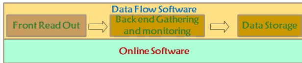
Fig. 3. Software architecture of DAQ.
