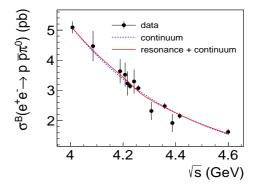
Figure 2: Fit to  $\sigma(e^+e^- \rightarrow p\bar{p}\pi^0)$  with resonance and continuum (solid line), or only continuum term (dashed line). Dots with error bars are the measured Born cross sections. The uncertainties are statistical only.
