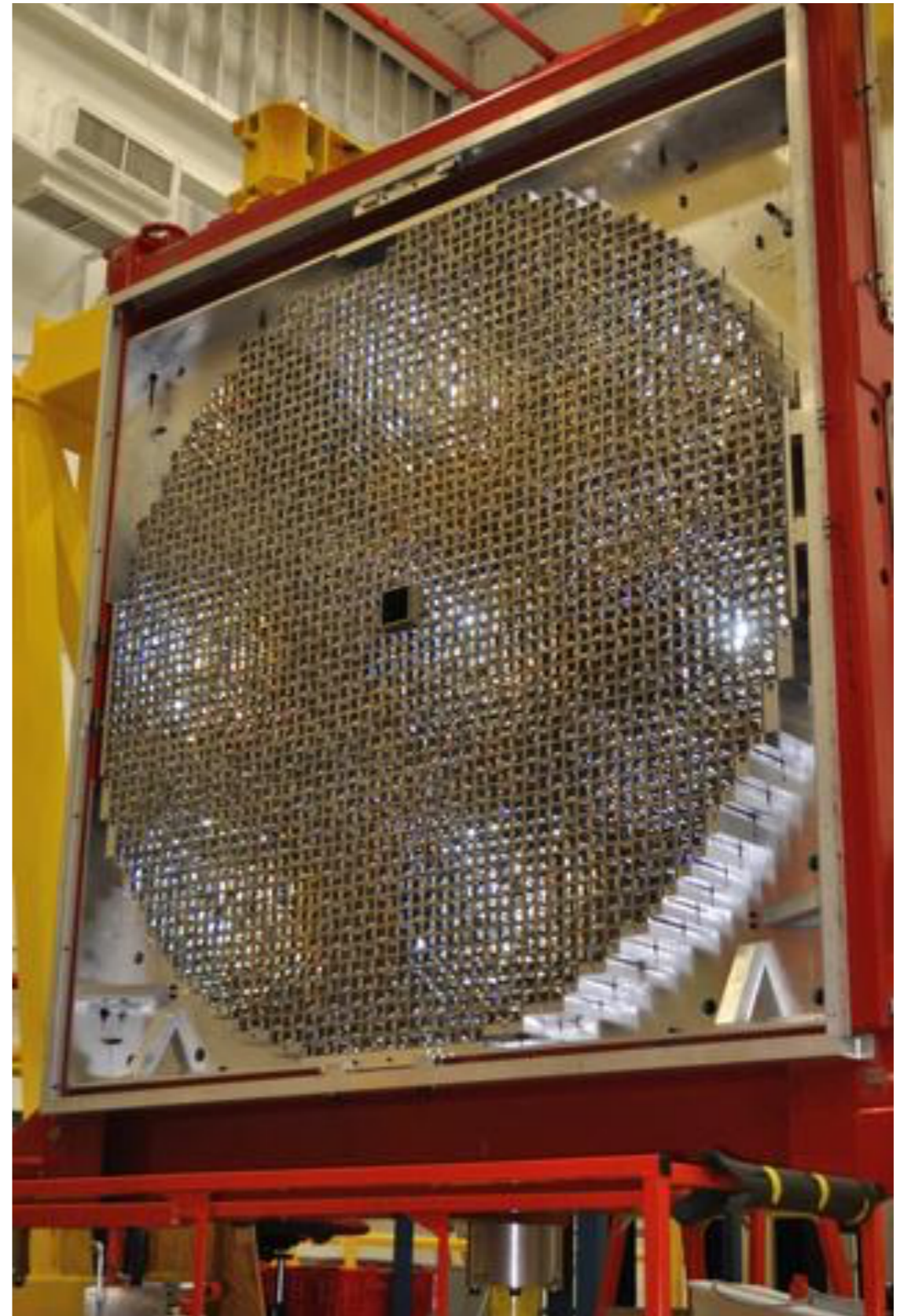
F8-00 lead glass, 4 \times 4 \times 45 cm
