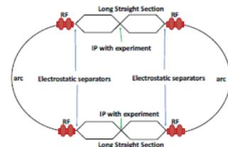
Figure 1: Schematic of the 'bowtie' idea (not to scale)
