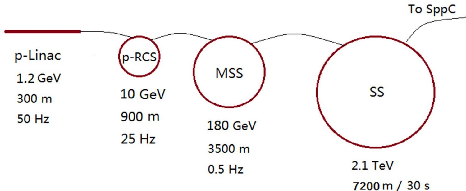
p-Linac: proton superconducting linac
