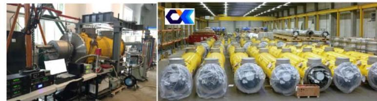
Fig. 6: IHEP ILC test cryomodule
