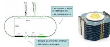
Fig. 9: ILC damping design and fast kiker
