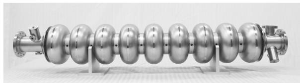
**TESLA cavity.** Nitrogen-doped bulk niobium and operates at 2 K.  $Q_0 > 3 \times 10^{10}$  at 24 MV/m for the vertical acceptance test.  $Q_0 > 1 \times 10^{10}$  up to 20 MV/m for long term operation.
