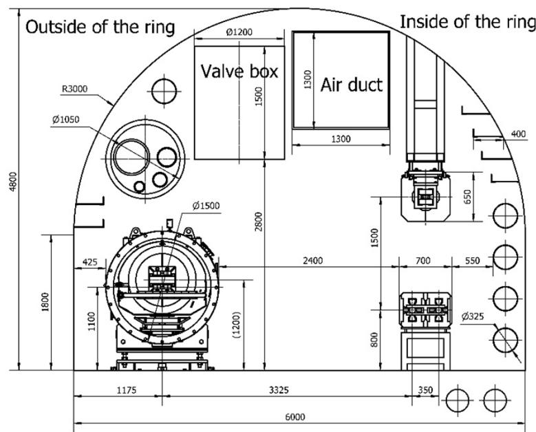
Tunnel cross section at RF-section
