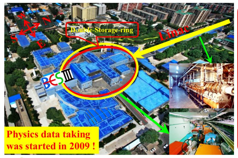
Beam energy: 1-2.3 GeV **Design Lum:** 1×10<sup>33</sup> cm<sup>-2</sup>s<sup>-1</sup> Opt. energy: 1.89 GeV **Energy spread:** 5.16 × 10<sup>-4</sup> **Bunches No.:** 93 **Bunch length:** 1.5 cm Total current: 0.91 A SR mode: 0.25A @ 2.5 GeV
