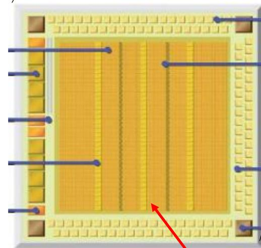
In the IC, there are many (huge amount of ) cells, and what we have to do is to connect the cells like making a road or route.
